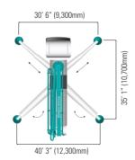
Front outrigger type X(Diagonal) Extension Rear outrigger type Swing-out
